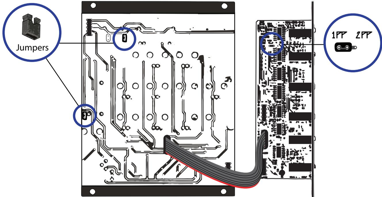
**BRAINS with a single PRESSURE POINT:** Use the single open "Close 4 Master" header, the BRAINS cable connected from "Points 1-4" header to EXPAND header, and the jumper on BRAINS set to "1PP."
