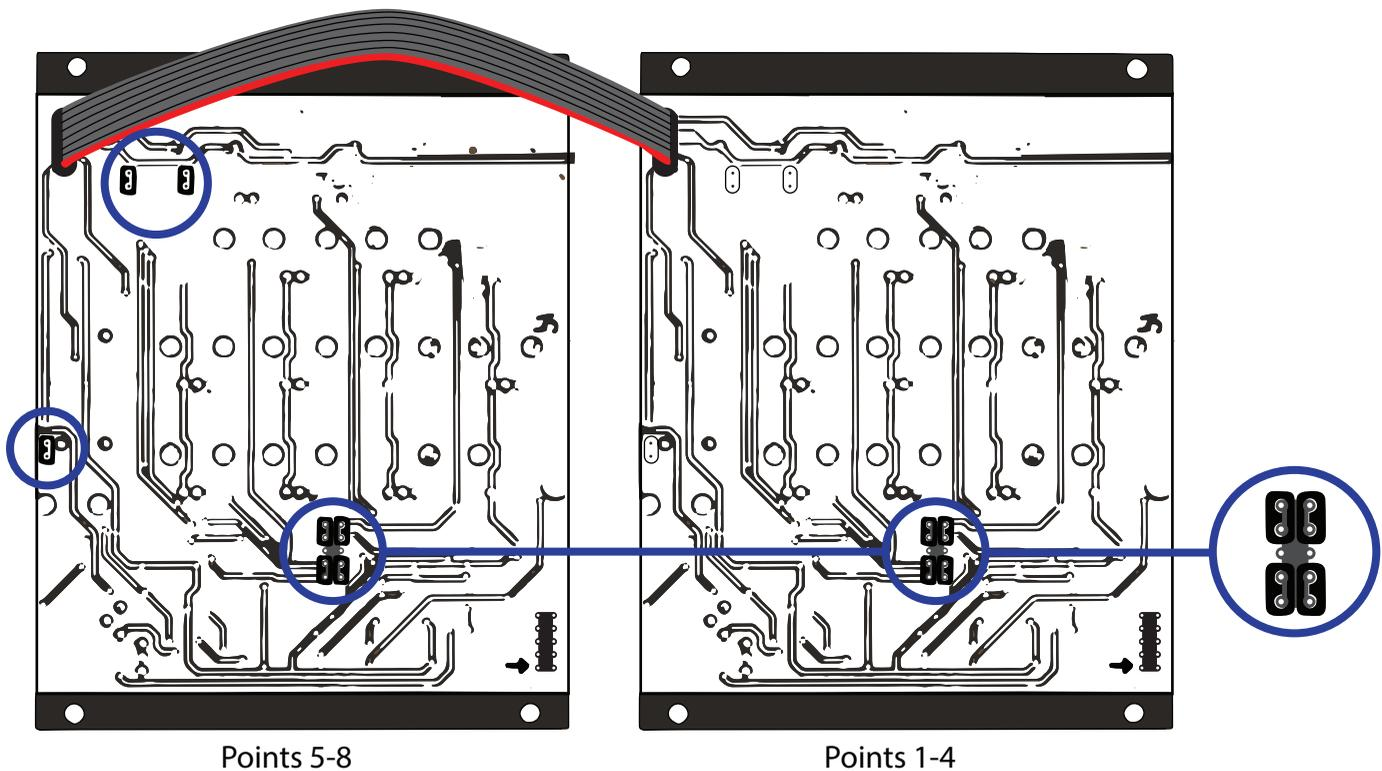
Two PRESSURE POINTS, chained: Note that the "Close 4 Master" headers are closed on the first unit (will be on the right when installed in the case). For three or four PRESSURE POINTS, use 4-header CHAIN cable and leave "Close 4 Master" headers open on all units but the master (rightmost when installed/leftmost from behind). Also, note the jumpers on the EXPAND headers.
