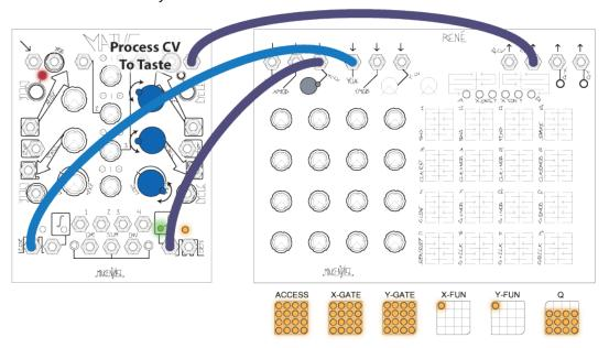
This feedback patch will cause Rene to jump locations every time it sends a CV value much greater than zero. Many nonlinear patterns await discovery. A "cluster" of higher CV values will cause extended sudden movement. "Eddies" can be created by setting several adjacent knobs to low values. Different clock sources in the X and Y clock inputs can create variation in the patterns.
